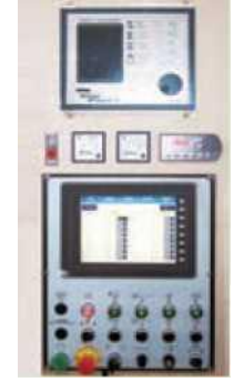
■ HMI Touch Screen, known as Human-Machine Interface, made in Japan (Optional Device). / Japon yapımı İnsan-Makine Arayüzü olarak bilinen İMA Dokunmatik Ekran, (Opsiyonel)
